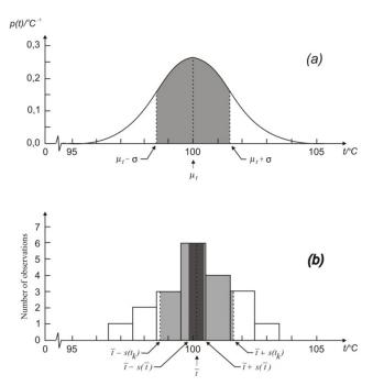
*Figure 2:* Graphical illustration of evaluating the standard uncertainty of an input quantity from repeated observations (Source; GUM, 1995)
