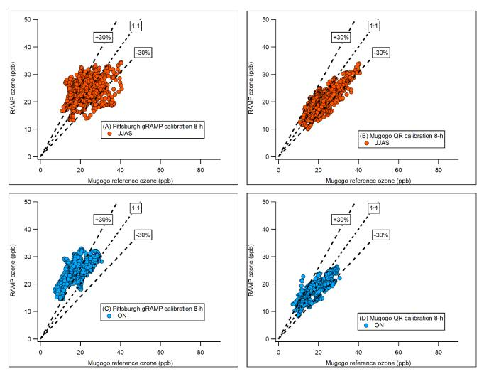
**Figure S2:** Comparison of RAMP calibration models for ozone with reference monitor data at the Mt Mugogo Climate Observatory. The "Pittsburgh gRAMP" model (A,C) is developed on collocations in Pittsburgh, PA, USA. The "Mugogo QR" model (B,D) is based on a collocation with the reference monitor at Mugogo; the data shown here includes both training (28 days) and testing (32 days) data. JJAS (A,B) is the dry season and ON (C,D) is the wet season.
