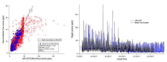
**Figure S4:** Ozone measurements in Kigali over the course of this study. (Left) Scatter plot shows most of the paired measurements across the city agree with each other. (Right) However, there are periods when the UR-CST O<sub>3</sub> is much higher than at Belle Vue estate.
