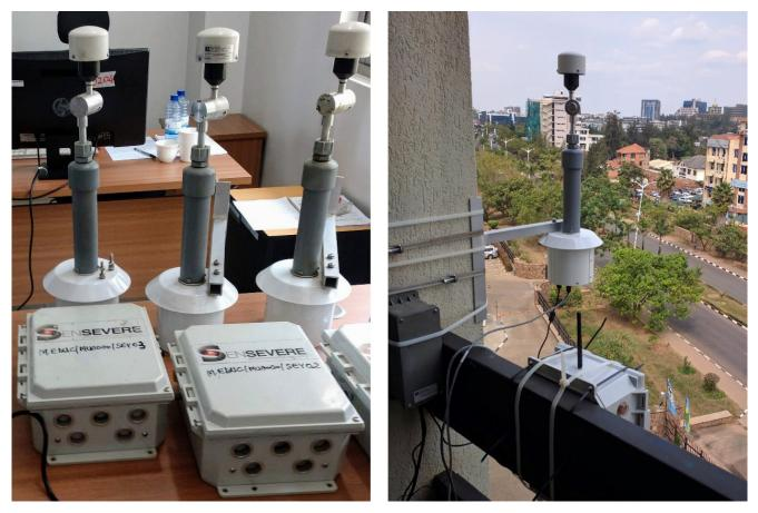
Figure S1: The RAMPs and the external Met-One NPMs in the lab (left) and a unit deployed in Kigali, Rwanda (right).
