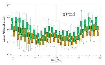
**Figure 5:** Diurnal variations in Angstrom Absorption Exponent (AAE) during the dry and wet seasons suggest vehicular emissions and domestic biofuel use contribute to ambient air pollution at different times of the day. The boxes show the IQR (25th and 75th percentiles of data); the notch shows the median; whiskers indicate the 9th and 91st percentiles. The corresponding hourly boxes for the two types of seasons are offset for visual clarity.
