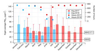
**Figure 2:** Monthly average PM<sub>25</sub> measured in Kigali over the course of this study. Red bars indicate 2017 and blue bars indicate 2018 data. Error bars are one standard deviation of the hourly measurements in that month. Solid round markers show the number of hourly data points collected in that month. Horizontal dashed lines indicate WHO annual guideline and the WHO's first interim target (IT 1).
