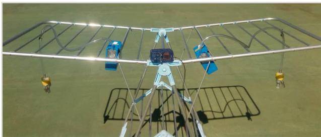
**Figure 2:** Sampling train on the rooftop showing the GilAir pumps, cyclone, and filter cassette.
